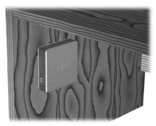
Figure 5-8 Thin client mounted under desk
